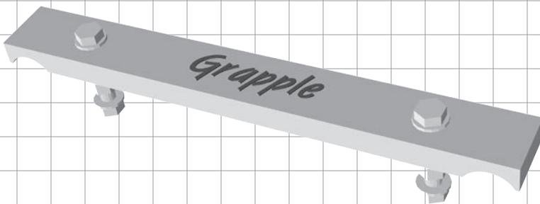
**The Grapple allows you to make inline 90 degree connections between similar trusses anywhere along a perpendicular primary truss. The load capacity of the inline truss will carry 75 percent of the manufacturer's load rating. The primary truss must have point load calculations taken into consideration. The secondary trusses must be supported at both ends. Cantilevering of truss is not recommended.**
