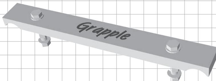
The Grapple allows you to make inline 90 degree connections between similar trusses anywhere along a perpendicular primary truss. The load capacity of the inline truss will carry 75 percent of the manufacturer's load rating. The primary truss must have point load calculations taken into consideration. The secondary trusses must be supported at both ends. Cantilevering of truss is not recommended.
